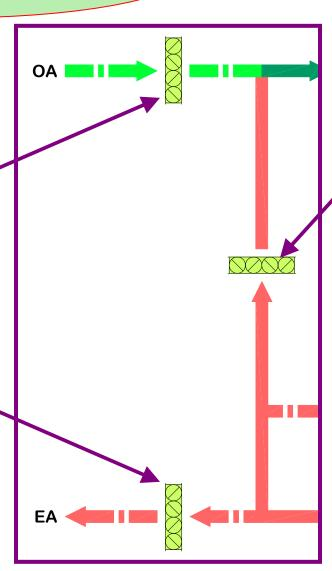
"Control Air Damper for Return Air " control return air capacity to adjust AC system
